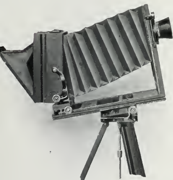
Fig. 3—Tilting bed reversed.
